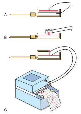
Figure 14-7. Principles of three types of electronic transducers for recording rapidly changing blood pressures (explained in the text).
