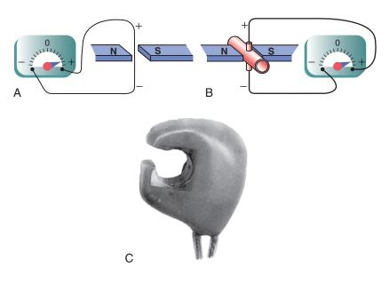
**Figure 14-4.** Flowmeter of the electromagnetic type, showing generation of an electrical voltage in a wire as it passes through an electromagnetic field (**A**); generation of an electrical voltage in electrodes on a blood vessel when the vessel is placed in a strong magnetic field and blood flows through the vessel (**B**); and a modern electromagnetic flowmeter probe for chronic implantation around blood vessels (**C**). N and S refer to the magnet's north and south poles.
