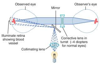
Figure 50-18. Optical system of the ophthalmoscope.
