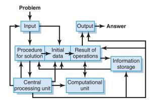
**Figure 46-4.** Block diagram of a general-purpose computer showing the basic components and their interrelations.
