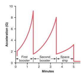
Figure 44-4. Acceleratory forces during takeoff of a spacecraft.
