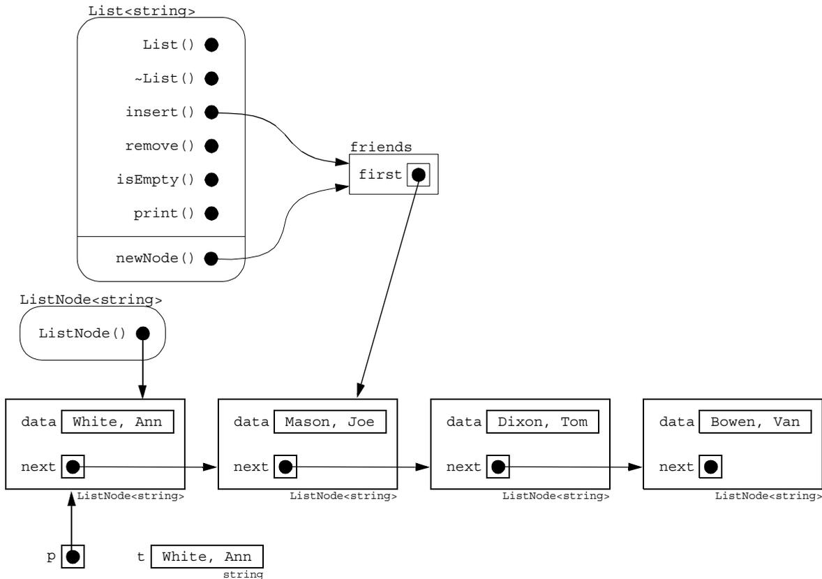
This shows the situation at the moment that the `insert()` function has invoked the `newNode()` function which has invoked the `ListNode()` constructor to create a new node for "White, Ann".
