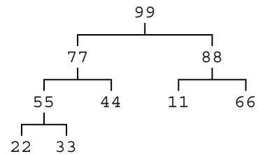
The `push_heap()` algorithm reverses the effect of `pop_heap()`. (See Example E.38.)
