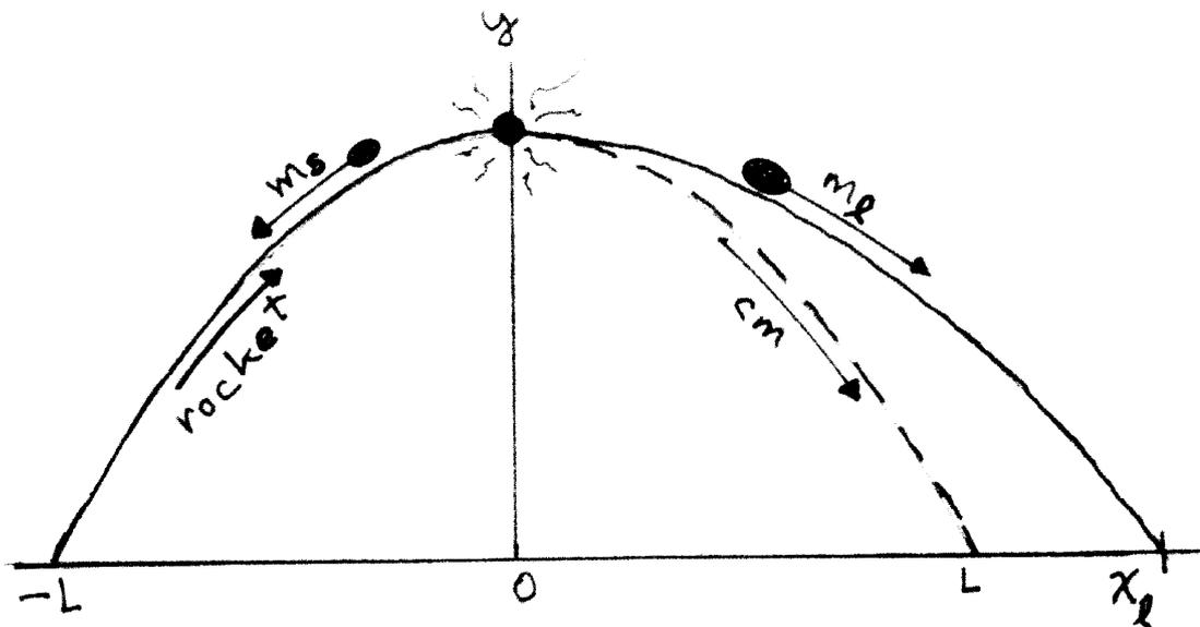
As long as the pieces are in flight, the center of mass continues on the parabolic trajectory. The time to rise is the same as the time to fall, so the center of mass reaches the ground at  $x = L$ . Let the smaller piece have mass  $m_s$ , and the larger piece have mass  $m_l$ , as indicated in the sketch.
