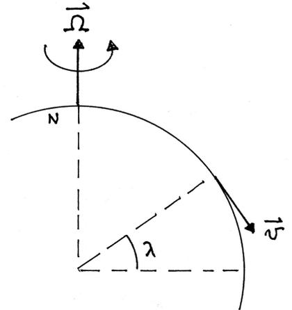
(b) From the sketch,  $\boldsymbol{\Omega} \times \mathbf{v}$  is directed into the page, toward the east. The Coriolis force on the train is directed toward the west, so the force on the tracks is toward the east. The Coriolis force vanishes at the equator, where  $\boldsymbol{\Omega} \times \mathbf{v} = 0$ .
