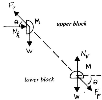
(b) The pole is taken to be massless, so the net force on the pole must be 0. The pole therefore exerts equal and opposite force  $F_p$  on each block, as indicated in the force diagrams. Consider only the equations of motion that do not involve the horizontal normal force  $N_h$  exerted on the upper block by the wall, and the vertical normal force  $N_v$  exerted on the lower block by the floor.
