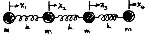
In the usual normal mode problem, the coupled equations of motion are solved for the frequencies, from which the relative amplitudes of the normal modes can be found. However, in a problem such as this that has a high degree of symmetry, the normal modes can be guessed, leading to the normal mode frequencies.
