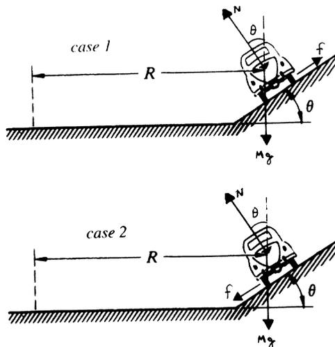
There are two cases, as the sketches indicate. Keep in mind that the friction force is opposed to the direction of motion. In case 1, the car will tend to slide down the slope if it is moving too slowly, so the friction force  $f$  is outward as shown. In case 2, the car will tend to slide up the slope if it is moving too fast, so  $f$  is inward.
