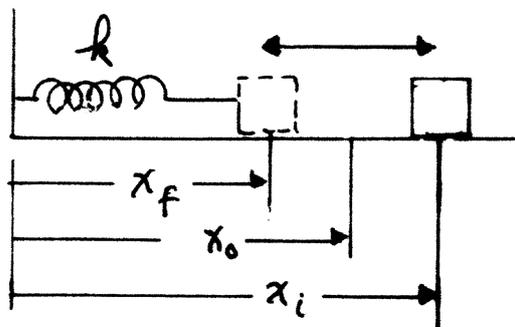
as shown. If there is no friction, the block returns to  $x_i$  after one complete cycle, and the mechanical energy is conserved.
