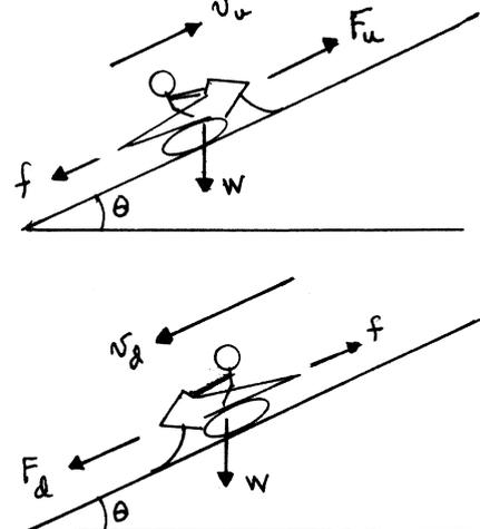
$F$  is the reaction force from the snow to the propelling force on the snow from the treads. The normal force on the snowmobile has no component along the slope, and is not shown in the sketches. The sketches are not to scale; according to the stated conditions, the slope angle  $\theta$  is  $\approx 1.4^\circ$ .
