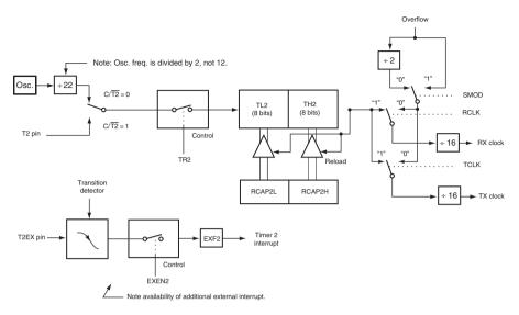
Figure C.16 Timer 2 in baud rate generator mode (courtesy Philips Semiconductors)
