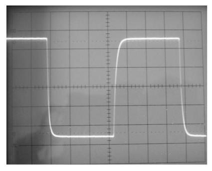
Figure 7.29(b) Function generator output response for square-waveform generation
