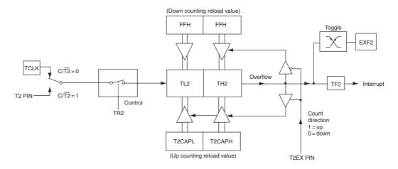
Figure F.12 Timer 2 auto-reload mode (DCEN =1) (courtesy Philips Semiconductors)
