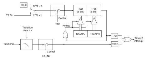
**Figure F.11** Timer 2 in auto-reload mode (DCEN = 0) (courtesy Philips Semiconductors)
