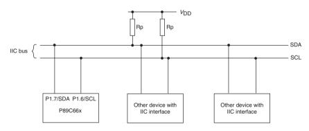
Figure D.15 Typical I<sup>2</sup>C bus configuration (courtesy Philips Semiconductors)
