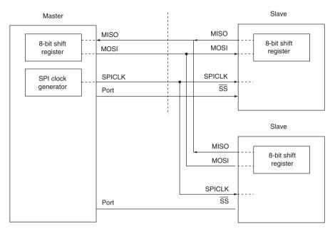
Figure E.8(c) SPI single master, multiple slaves configuration (courtesy Philips Semiconductors)
