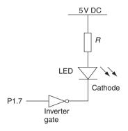
Figure 1.6 Use of an LED to indicate the state of port 1, pin 7
