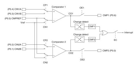
Figure E.9 Comparator input and output connections (courtesy Philips Semiconductors)
