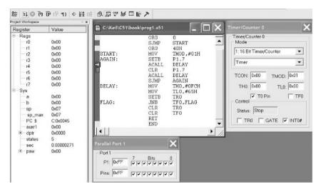
Figure 4.6 Simulation display showing the use of breakpoints
