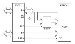
Figure C.5 Use of external program memory (courtesy Philips Semiconductors)
