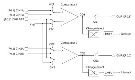
Figure 5.12 Comparator configurations of the 87LPC769 microcontroller
