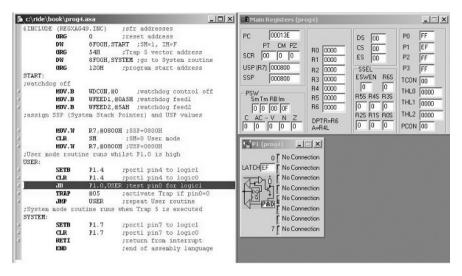
Figure 6.13 Simulation response showing the effect on system registers of a trap interrupt
