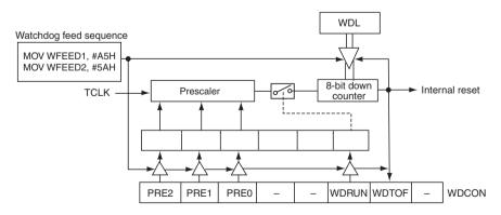
Figure F.13 XAG49 watchdog timer arrangement (courtesy Philips Semiconductors)
