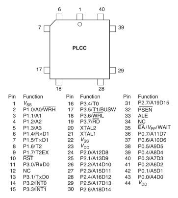
Figure 2.9 Pin functions for the XAG49 PLCC package microcontroller
