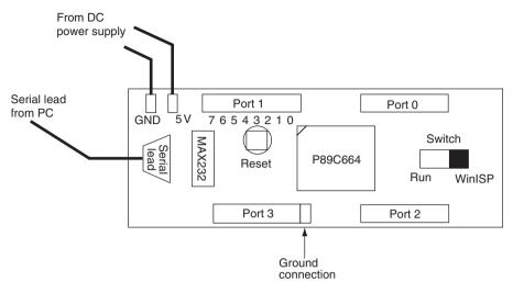
Figure 2.4(b) Diagram of the 89C66x microcontroller board showing ports, switches and external connections
