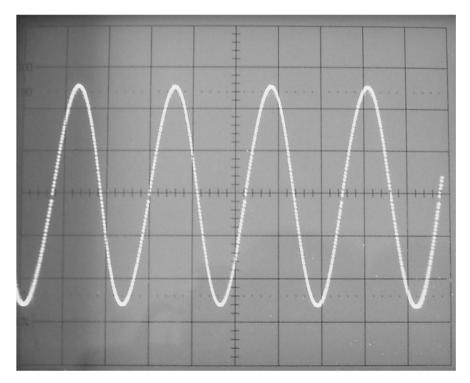
Figure 7.29(a) Function generator output response for sine waveform generation
