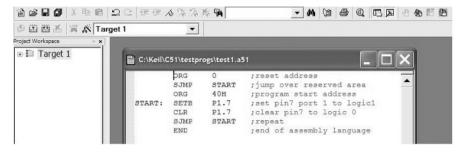
Figure 3.9 Text window showing test1.a51 source program
