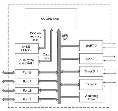
Figure F.1 XAG49 block diagram (courtesy Philips Semiconductors)
