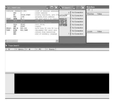
Figure 3.46 Trace window for test1.axa program
