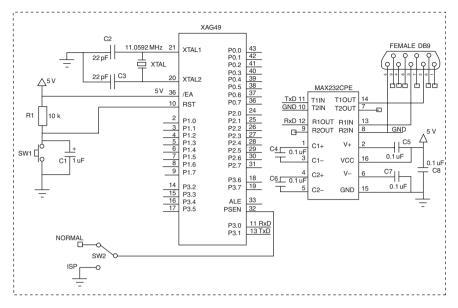
Figure 2.10 Schematic for the XAG49 microcontroller board
