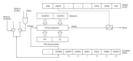
Figure D.12 PCA watchdog timer m (module 4 only) (courtesy Philips Semiconductors)
