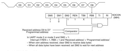
Figure D.14 UART multiprocessor communication, automatic address recognition (courtesy Philips Semiconductors)
