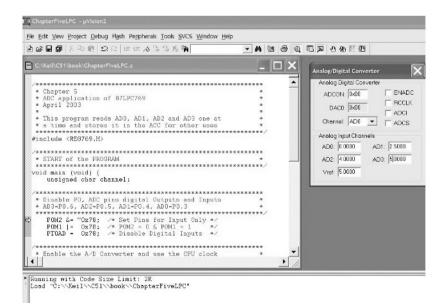
Figure 5.9 Changing the values of the analog input channels
