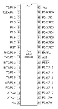
Figure C.2 80C51 pin-out layout (courtesy Philips Semiconductors)
