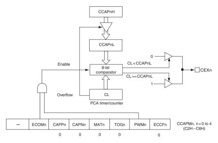
Figure D.11 PCA PWM mode (courtesy Philips Semiconductors)
