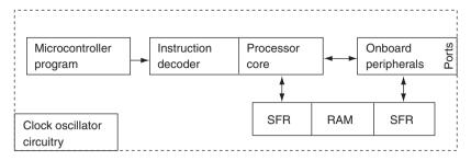
Figure 1.4 Block diagram of a microcontroller
