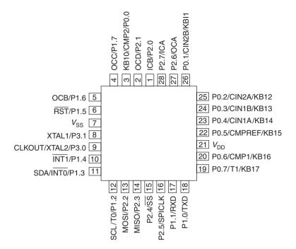
Figure E.2 PLCC 28-pin package (courtesy Philips Semiconductors)
