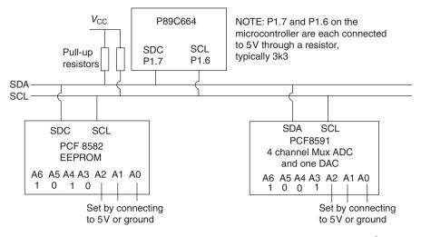
Figure 4.33 P89C664 microcontroller connected to slave devices via the I<sup>2</sup>C bus
