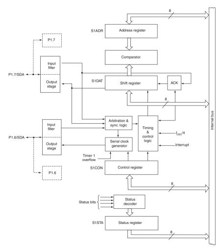
Figure D.17 I<sup>2</sup>C bus serial interface block diagram (courtesy Philips Semiconductors)
