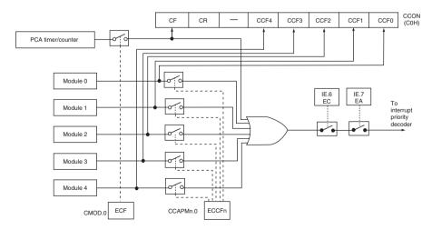
Figure D.7 PCA interrupt system (courtesy Philips Semiconductors)
