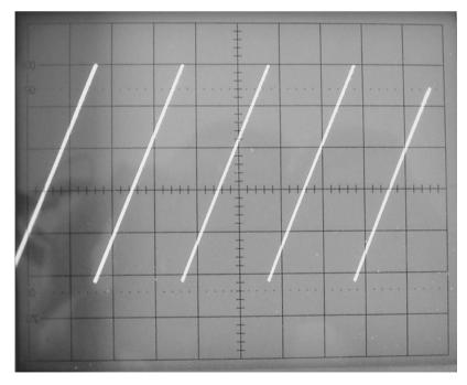
Figure 7.29(c) Function generator output response for sawtooth waveform generation
