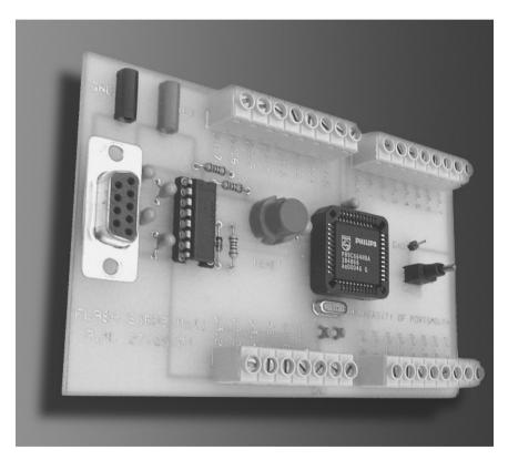
Figure 2.4(a) The 89C66x microcontroller board
