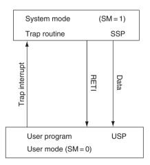
Figure 6.12 Use of trap interrupts
