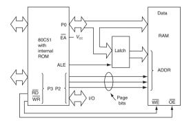
Figure C.7 Access of external data memory (courtesy Philips Semiconductors)
