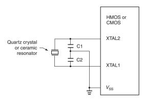
Figure C.20 80C51 on-chip oscillator (courtesy Philips Semiconductors)
