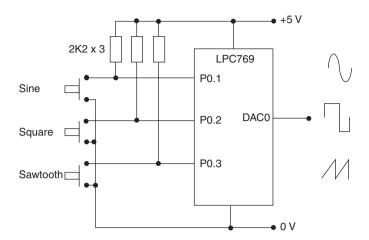
Figure 7.24 Block diagram of function generator using a P87LPC769 microcontroller
