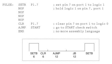
**Figure 1.12** Waveform produced using specified instructions. Note that the waveform is not a square wave (i.e. there are unequal ON and OFF periods)
