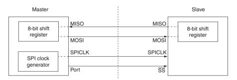
Figure 5.15 Simple master and slave connection
