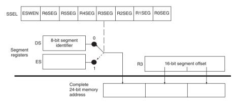
Figure F.6 Use of segment registers for XA address generation (courtesy Philips Semiconductors)
