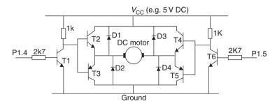
Figure 7.3 A bridge drive circuit using the inputs from port pins P1.4 and P1.5 to control the DC motor speed and direction of rotation
