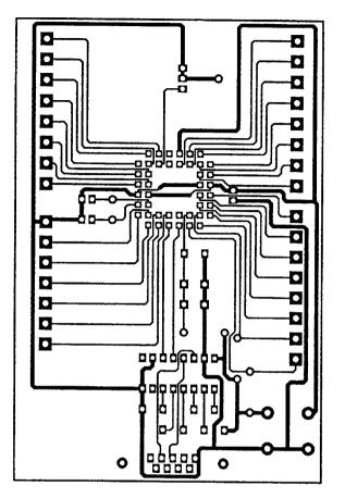
Figure G.3 Full-size single-sided artwork for the XAG49 microcontroller board
