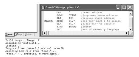
Figure 3.16 Creation of a hex file for test1.a51 program
