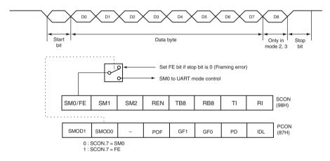
Figure C.18 UART framing error detection (courtesy Philips Semiconductors)
