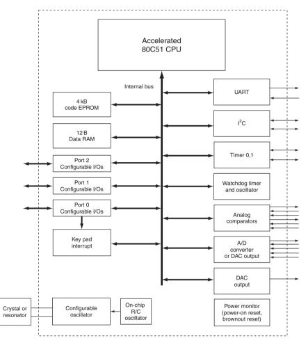
Figure 5.1 Block diagram of the 87LPC769 microcontroller
