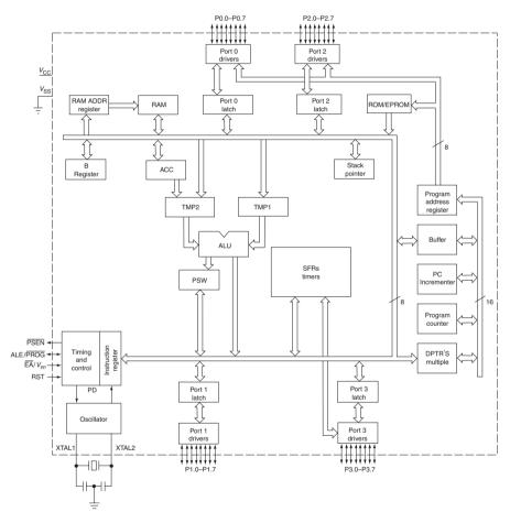
Figure C.1 80C51 block diagram (courtesy Philips Semiconductors)
