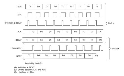
Figure D.19 Shift-in and shift-out timing (courtesy Philips Semiconductors)
