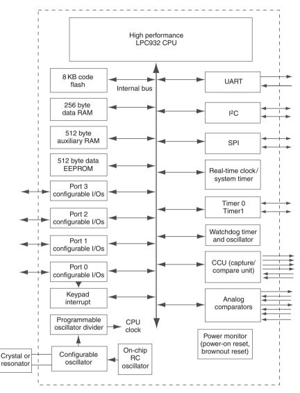
Figure E.1 LPC932 block diagram (courtesy Philips Semiconductors)
