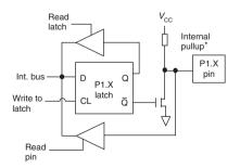
Figure C.9 80C51 port 1 bit latch (courtesy Philips Semiconductors)
