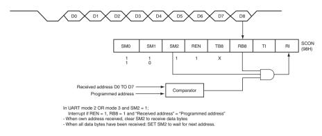
Figure C.19 UART multiprocessor communication, automatic address recognition (courtesy Philips Semiconductors)
