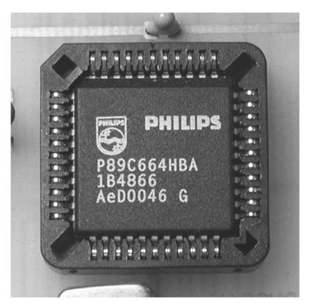
Figure 1.1 Philips P89C664 PLCC package microcontroller
