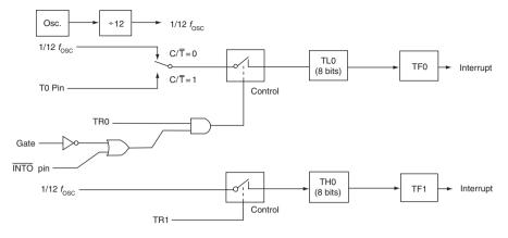
Figure C.12 Timer/counter 0 mode 3 configuration (courtesy Philips Semiconductors)
