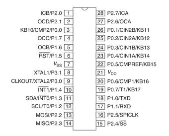
Figure 5.14 Pin configuration for the 89LPC932 microcontroller
