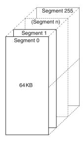
Figure F.5 XA data memory segments (courtesy Philips Semiconductors)
