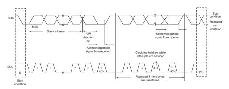
Figure D.16 Data transfer on the I<sup>2</sup>C bus (courtesy Philips Semiconductors)
