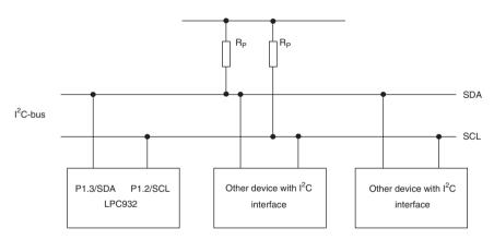
Figure E.7 I<sup>2</sup>C bus configuration (courtesy Philips Semiconductors)
