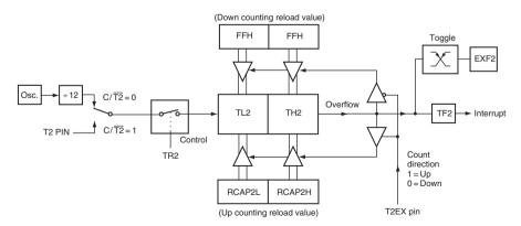
Figure C.15 Timer 2 in auto-reload mode (DCEN = 1) (courtesy Philips Semiconductors)
