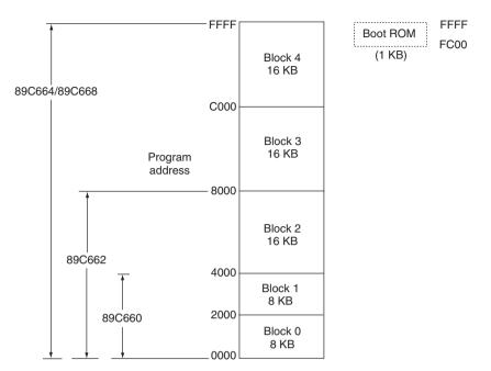
Figure D.4 Flash memory configurations (courtesy Philips Semiconductors)
