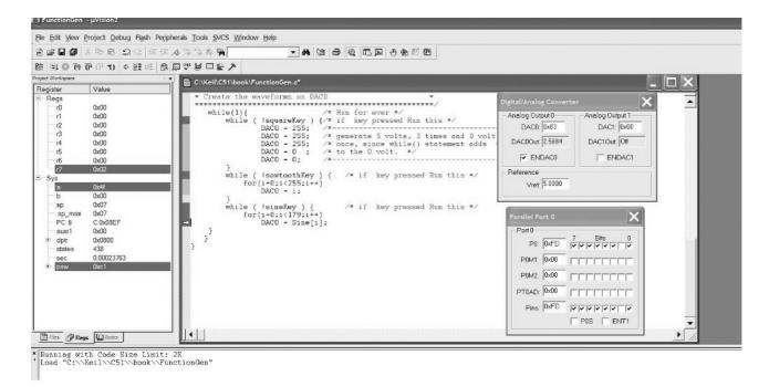
Figure 7.26 Simulation window, with the DAC0 and port 0 windows added, for sine waveform generation
