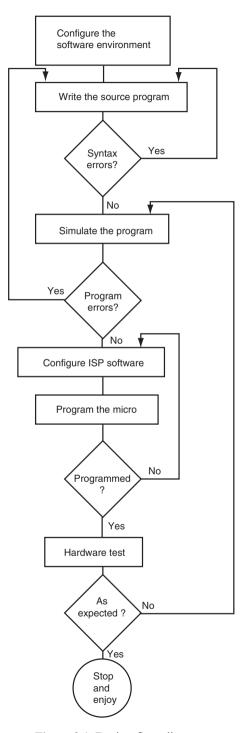
Figure 3.1 Design flow diagram
