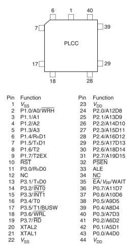
Figure F.2 XAG49 PLCC package pin-out layout (courtesy Philips Semiconductors)
