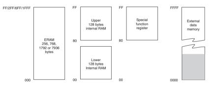
Figure D.3 89C66x internal/external data memory address spaces (courtesy Philips Semiconductors)
