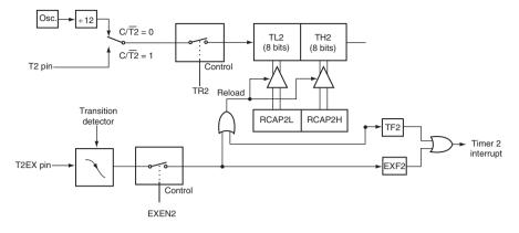
Figure C.14 Timer 2 in auto-reload mode (DCEN = 0) (courtesy Philips Semiconductors)
