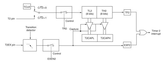
Figure F.10 Timer 2 in capture mode (courtesy Philips Semiconductors)
