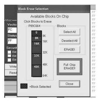
Figure 2.6 Block erase selection using WinISP
