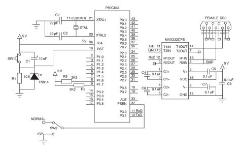
Figure 2.2 Schematic for the 89C66x microcontroller board
