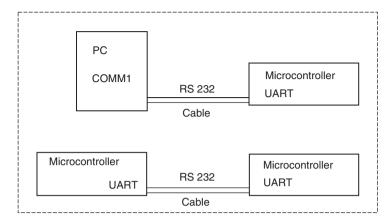
Figure 4.25 Use of RS232 interface between PC and microcontroller or between two microcontrollers
