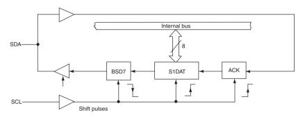
Figure D.18 Serial input/output configuration (courtesy Philips Semiconductors)
