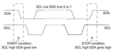
Figure 4.34 Data transfer on the I<sup>2</sup>C bus
