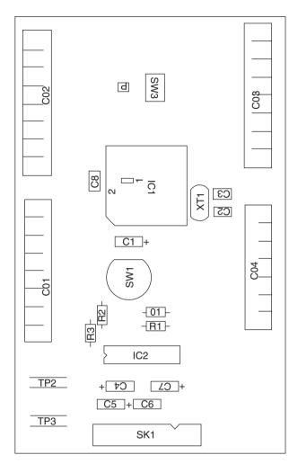
Figure G.2 Component layout for the P89C66x microcontroller board
