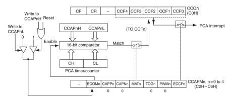
Figure D.9 PCA compare mode (courtesy Philips Semiconductors)
