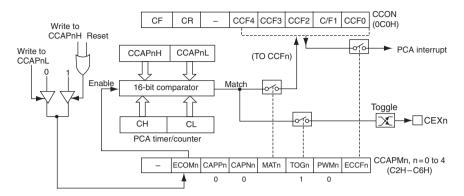
Figure D.10 PCA high-speed output mode (courtesy Philips Semiconductors)
