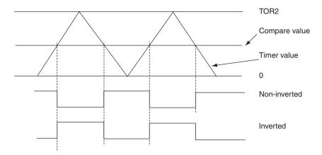
Figure E.4 Symmetrical PWM waveform (courtesy Philips Semiconductors)
