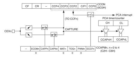
Figure D.8 PCA capture mode (courtesy Philips Semiconductors)
