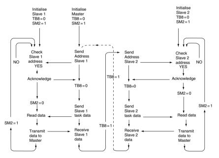
Figure 7.20 Communication protocol for master/slave communication
