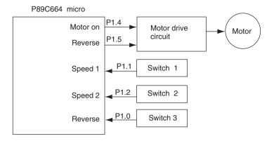
Figure 7.1 Block diagram for speed control of a small DC motor using a P89C664 microcontroller
