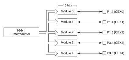
Figure 4.16 Programmable counter array (PCA)
