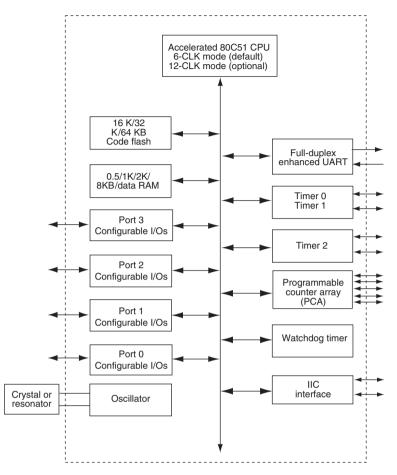
Figure D.1 89C66x block diagram (courtesy Philips Semiconductors)
