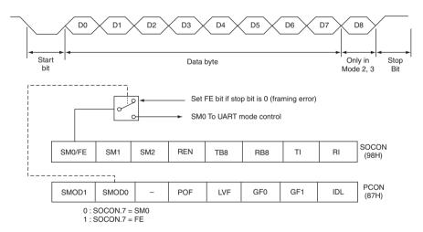
Figure D.13 UART framing error detection (courtesy Philips Semiconductors)
