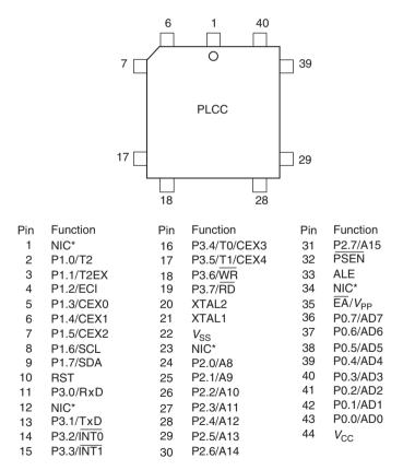
Figure 2.1 Pin functions for the 89C66x PLCC package microcontroller
