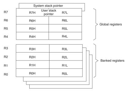
Figure F.3 XA register file diagram (courtesy Philips Semiconductors)
