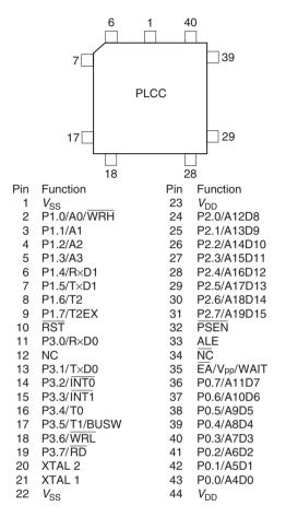
Figure 6.17 Pin functions for the XAG49 PLCC package
