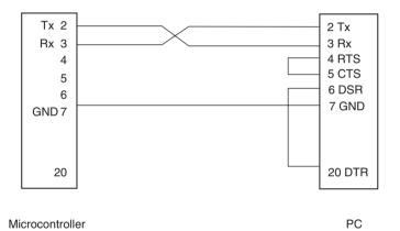
Figure 4.26 RS 232 transmit (Tx) and receive (Rx) connections between a PC and microcontroller
