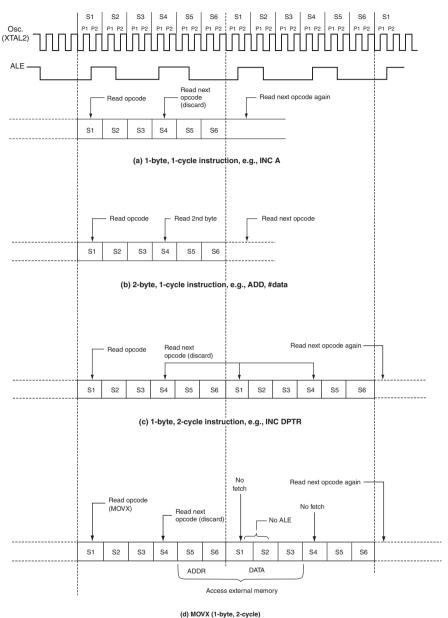
Figure C.22 80C51 family state sequences (courtesy Philips Semiconductors)
