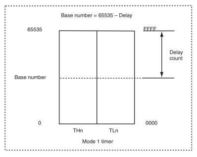
Figure 4.3 Determination of delay count for a mode 1 timer
