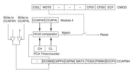
Figure 4.21 Use of module 4 of the PCA to facilitate the watchdog timer
