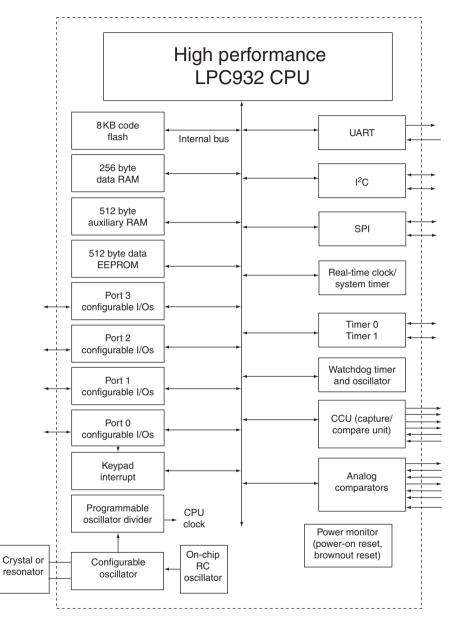
Figure 5.13 Block diagram of the 89LPC932 microcontroller
