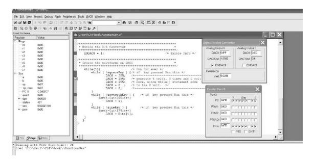
Figure 7.27 Simulation window, with the DAC0 and port 0 windows added, for square-waveform generation
