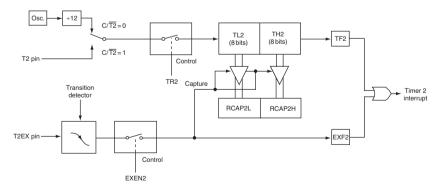
Figure C.13 Timer 2 in capture mode (courtesy Philips Semiconductors)
