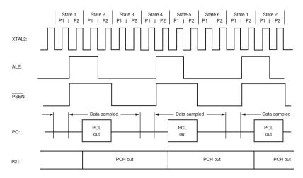
Figure C.6 External memory program fetches (courtesy Philips Semiconductors)
