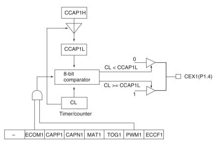
Figure 4.18 Use of the PCA to produce a PWM output from port 1, pin 4
