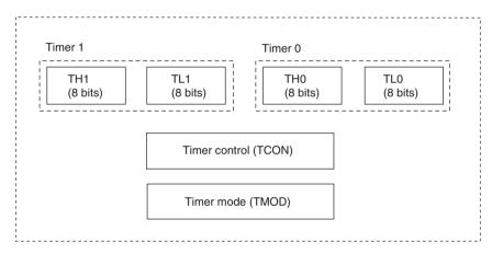
Figure 4.1 Timer 0/1 arrangement for the 89C66x family
