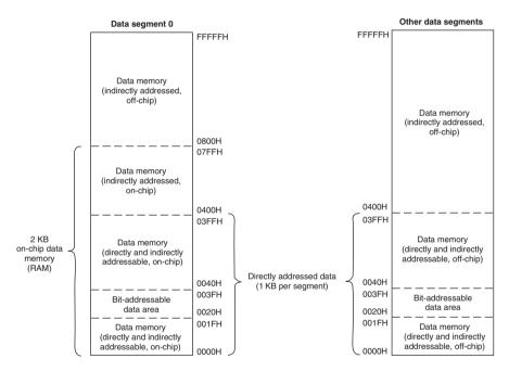
Figure F.7 XAG49 data memory map (courtesy Philips Semiconductors)
