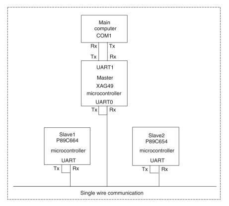
Figure 7.19 Block diagram of a single wire communication system
