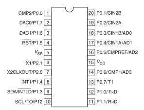
Figure 5.2 Pin configuration for the 87LPC769 microcontroller
