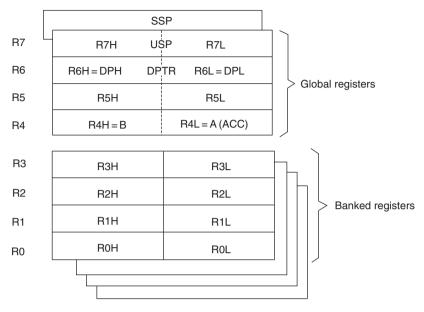
Figure 6.10 XAG49 general-purpose registers
