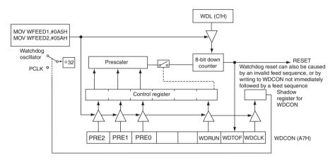
**Figure E.5** Watchdog timer in watchdog mode (WDTE = 1) (courtesy Philips Semiconductors)
