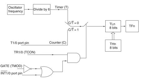
Figure 4.8 Circuit for timer 1/0 to operate as an 8-bit up-counter in mode 2
