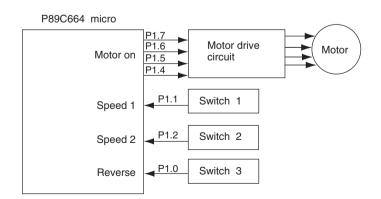
Figure 7.7 Block diagram for speed control of a stepper motor using a P89C664 microcontroller
