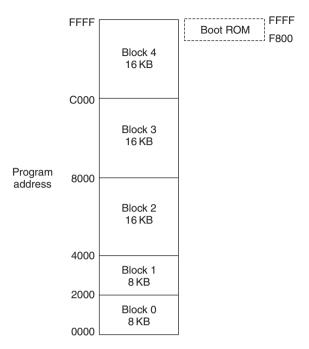
Figure F.9 XAG49 flash memory configuration (courtesy Philips Semiconductors)
