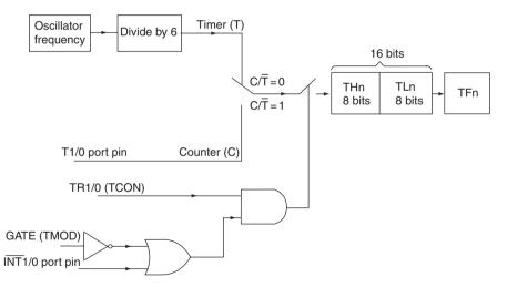
Figure 4.2 Circuit for timer 0/1 operating as a 16-bit up-counter in mode 1
