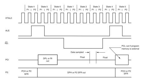
Figure C.8 External data memory read cycle (courtesy Philips Semiconductors)
