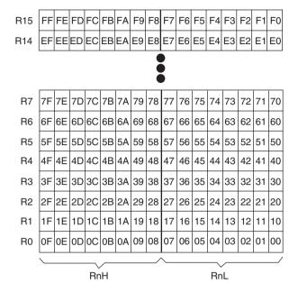
Figure F.4 XA bit address to registers (courtesy Philips Semiconductors)
