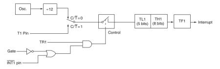
Figure C.10 Timer/counter mode 0 configuration (courtesy Philips Semiconductors)
