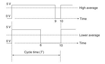
Figure 4.17 Waveforms showing the effect of pulse width modulation (PWM) in varying the average DC voltage over a cycle period (T)
