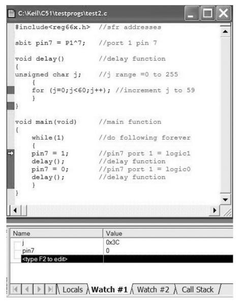
Figure 3.27 C language program to produce toggling on pin 7, port 1 with a time delay
