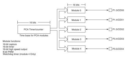
Figure D.5 Programmable counter array (PCA) (courtesy Philips Semiconductors)
