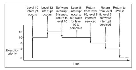
Figure 6.16 Example illustrating event and software interrupt prioritising
