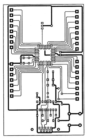
Figure G.1 Full-size single-sided artwork for the P89C66x microcontroller board
