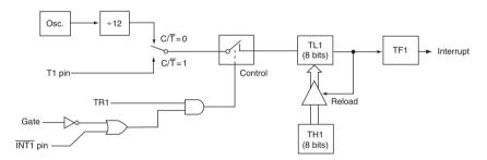
Figure C.11 Timer/counter mode 2 configuration (courtesy Philips Semiconductors)
