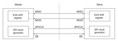
Figure E.8(b) SPI dual device configuration, where either device can be master or slave (courtesy Philips Semiconductors)
