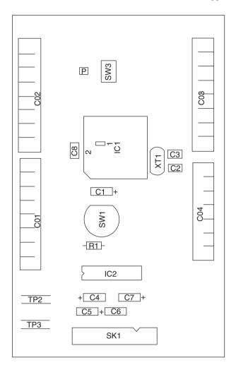
Figure G.4 Component layout for the XAG49 microcontroller board
