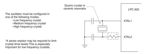
Figure E.10 Using the crystal oscillator (courtesy Philips Semiconductors)
