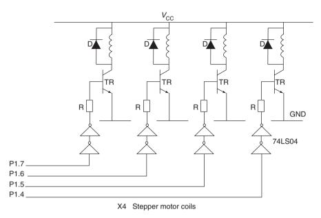
Figure 7.9 Suitable circuit arrangement to provide a drive for a stepper motor
