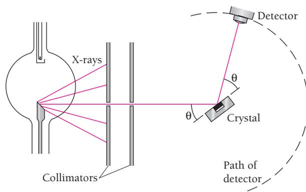
Figure 2.21 X-ray spectrometer.
