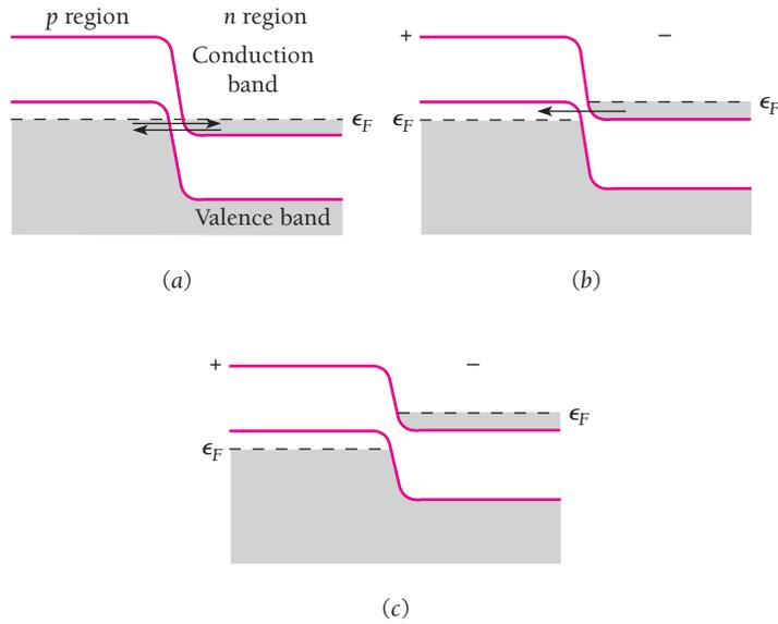
**Figure 10.33** Operation of a tunnel diode. (a) No bias. Electrons tunnel both ways between the *p* and *n* regions. (b) Small forward bias. Electrons tunnel from the *n* to the *p* region only. (c) Larger forward bias. Now the valence band of the *p* region does not overlap the conduction band of the *n* region and so no tunneling can occur. At higher voltages the diode behaves like the ordinary diode of Fig. 10.30.
