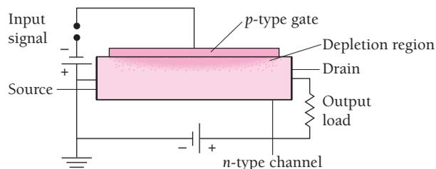
**Figure 10.38** A field-effect transistor.
