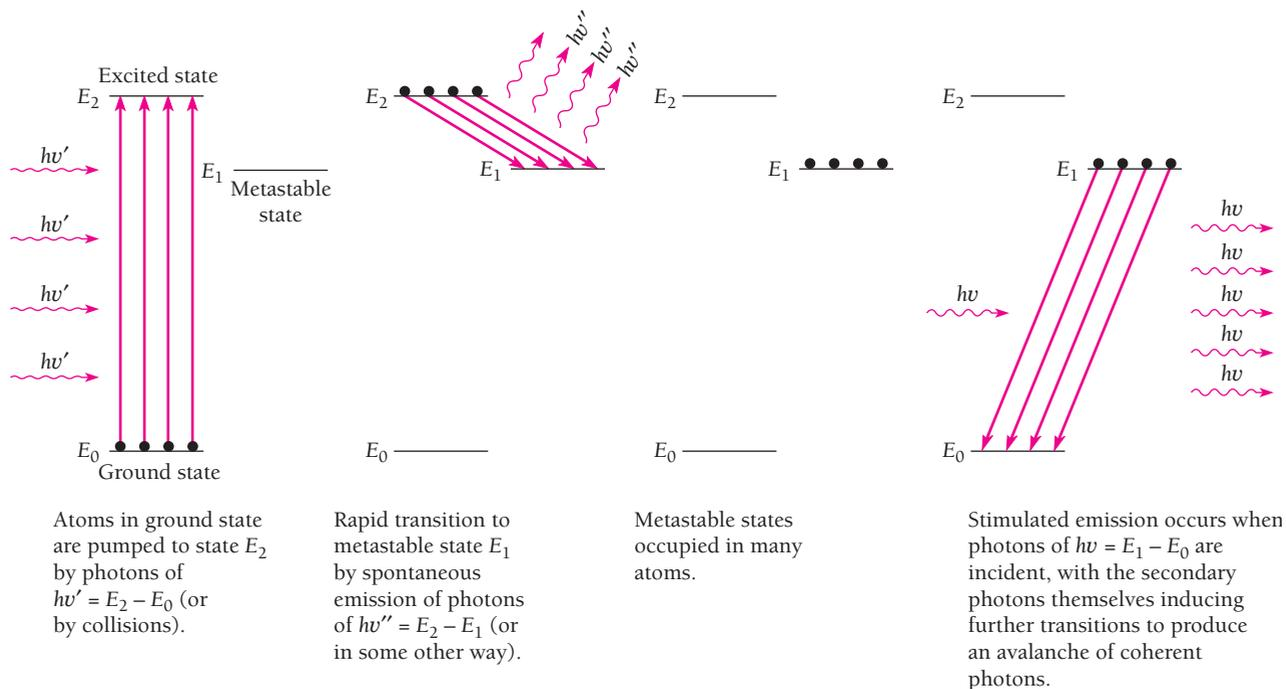
Figure 4.26 The principle of the laser.
