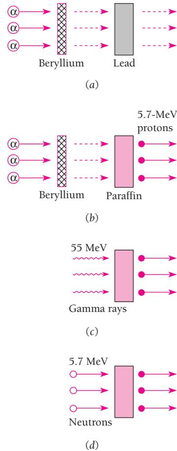
**Figure 11.2** (a) Alpha particles incident on a beryllium foil cause the emission of a very penetrating radiation. (b) Protons of up to 5.7 MeV are ejected when the radiation strikes a paraffin slab. (c) If the radiation consists of gamma rays, their energies must be at least 55 MeV. (d) If the radiation consists of neutral particles of approximately proton mass, their energies need not exceed 5.7 MeV.
