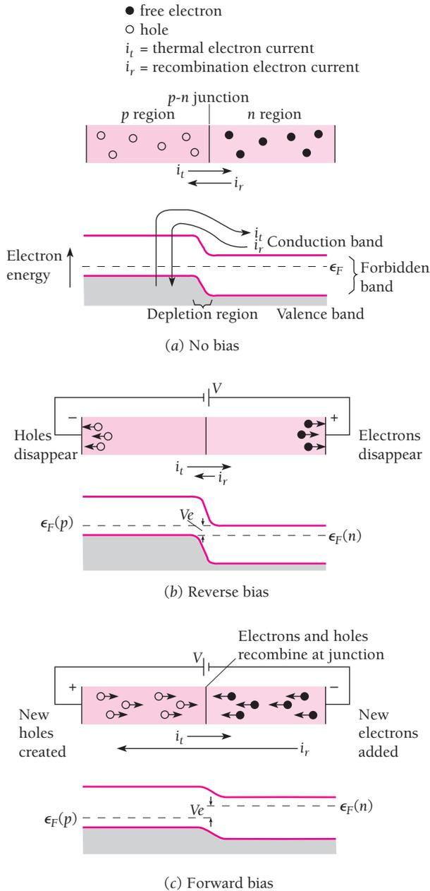
**Figure 10.30** Operation of a semiconductor diode.
