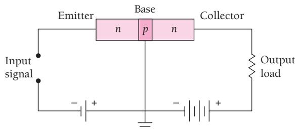
Figure 10.36 A simple junction-transistor amplifier.
