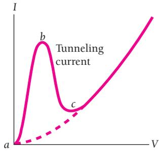
**Figure 10.34** Voltage-current characteristic of a tunnel diode. The points *a*, *b*, and *c* correspond to parts *a*, *b*, and *c* of Fig. 10.33. The dashed line indicates the behavior of an ordinary junction diode, as in Fig. 10.30.
