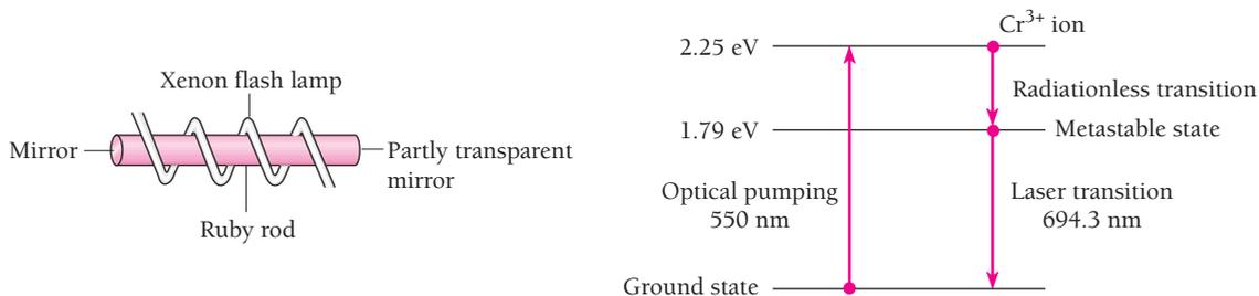
Figure 4.27 The ruby laser. In order for stimulated emission to exceed stimulated absorption, more than half the Cr<sup>3+</sup> ions in the ruby rod must be in the metastable state. This laser produces a pulse of red light after each flash of the lamp.
