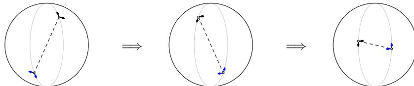
At the end of the circuit, the  $x$  part of the  $xy$ -axes sticks out in the other direction. Thus, in the projective plane we cannot describe a figure as right- or
