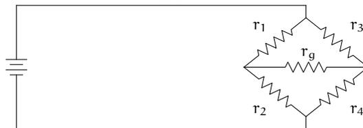
$r_2/r_1$  equals  $r_4/r_3$  if and only if the current flowing through  $r_g$  is zero. (In practice, we place an unknown resistance at  $r_4$ . At  $r_g$  we place a meter that shows the current. We vary the three resistances  $r_1$ ,  $r_2$ , and  $r_3$  (typically they each have a calibrated knob) until the current in the middle reads 0, and then the above equation gives the value of  $r_4$ .)
